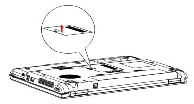
Figure 8-5 Removing the cover
